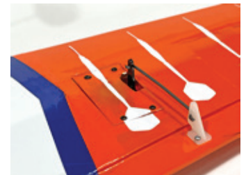
Sample control horn and pushrod installation for ailerons
