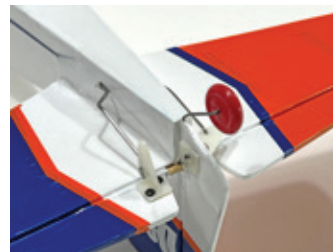
Sample control horn and pushrod installation for elevator and rudder
