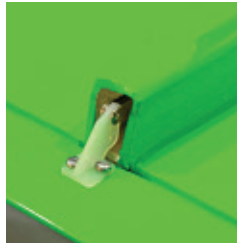
Elevator pushrod exits out the rear of the fuselage
