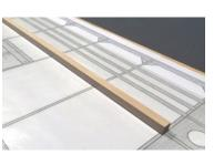
of medium CA instead of t-pins. Be sure it is aligned properly and is straight over it's entire length. The alignment of this spar is critical as the rest of the wing panel is based off this single piece.
