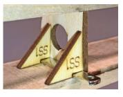
be positioned so the end with the 2 closer holes is inside the wing, and the other end protruding from the bottom wing's surface by a 1/4" to 3/8". It also should rest flat against the sheer web and be up against the R7 rib.
