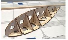
Then gently slide this sub-assembly into the notches in the R8A/B assembly from the last step. When satisfied with the fit, glue them together.
