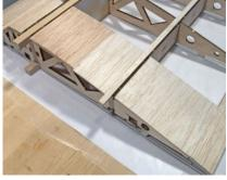
Working on one section at a time, and note that the center gap (between the main spar and the rear sub-spar) will require a couple 1/16th pieces to be edge joined together to cover the gap.
