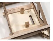
Now fit the servo hatches into position on the bottom of the wing. Using the pre-cut holes as a guide, drill four 1/16'' mounting holes into the  $3/16'' \times 3/8''$  basswood mounting strips installed earlier. Harden the wood with a bit of thin CA and you can use the supplied  $2-56 \times 3/4''$  self tapping screws to secure them in place.
