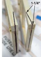
will taper correctly. Although you can cut this with a saw or hobby knife, sandpaper makes quick work of this, but use caution not to remove too much.
