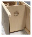
sanding to fit, glue it to the front of F2 to complete the thickened firewall. Use epoxy for this step and be sure to firmly clamp this piece in position while the glue cures.
