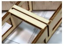
We recommend dry-fitting these first, then gluing together. Try to keep glue out of the slot in G1 as this is where the main landing gear will be mounted.
