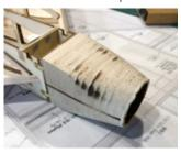
Now, to hold the cowl in position, drill into the holes in each cowl mounting tab using a 1/16" bit. Make the holes about a 1/2" deep. Using 4 of the supplied 2-56 x 3/4" self tapping screws, attach the cowl to the Comet.
