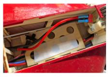
For electric power, locate TF from LP3. This can be glued in place and used as the "floor" to mount the flight battery to using a bit of hook-and-loop (not included).
