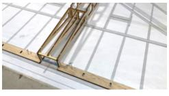
as shown on the plans, over the trailing edge. Use a long straight edge to assure that both edges line up. The inner notch will fit around the extended tab on the back of the R1 pieces.
