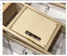
The next steps involve assembling and attaching the firewall.
