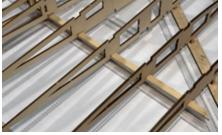
plans. Take time to measure correctly before cutting. Starting with the outside rib (R5), slide each spar in position into the pre-cut pocket on the bottom of each rib. Be careful that you do not break off the tabs as they are used to hold these spars in position.
