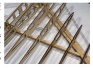
When satisfied with the alignment, glue the front and rear spars in place, making sure they are attached to all of the ribs and to each other.
